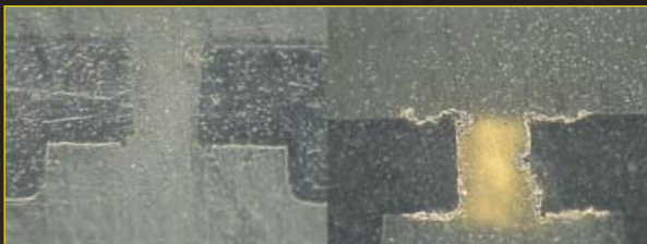
Figure 2 shows a cross-section through a 300 \mu\text{m} through-plating (via), magnified 100 times, before and after the metal coating.
