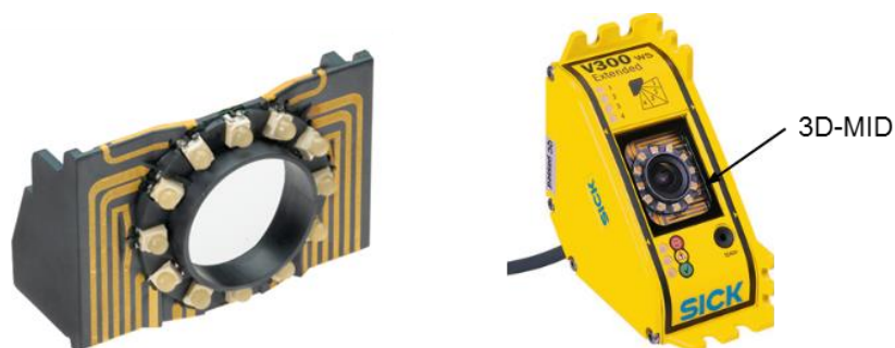
Fig. 3: 3D-MID lighting module (left side) and integrated in the camera system (right side)
