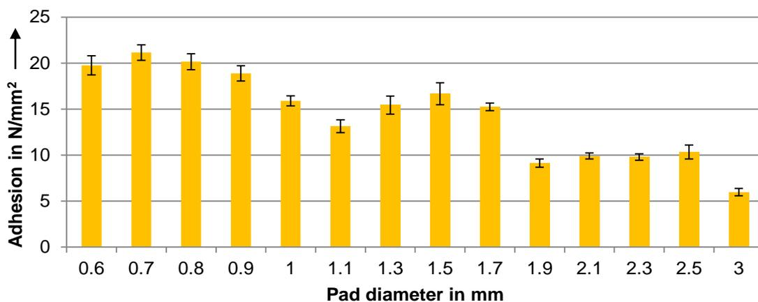
Fig. 3: Evaluation of the hot pin pull test for pad diameters from 0.6 mm to 3.0 mm
