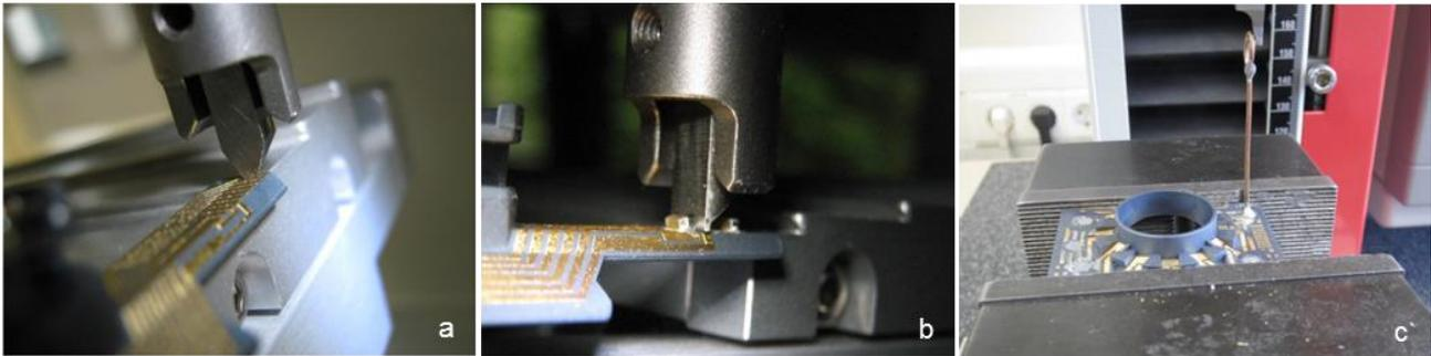
Fig. 1: Shear test of circuit tracks (a) or electronic components (b) and pull-off test (c)
