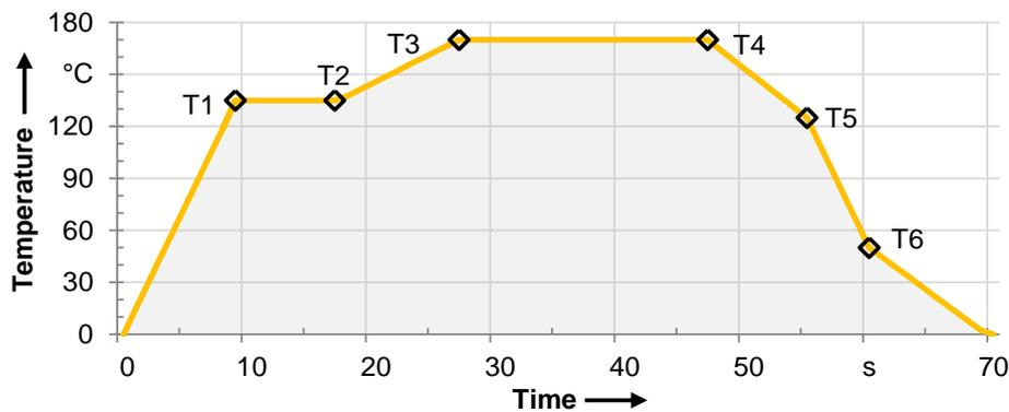
Fig. 4: Temperature profile with a peak temperature of 170 °C
