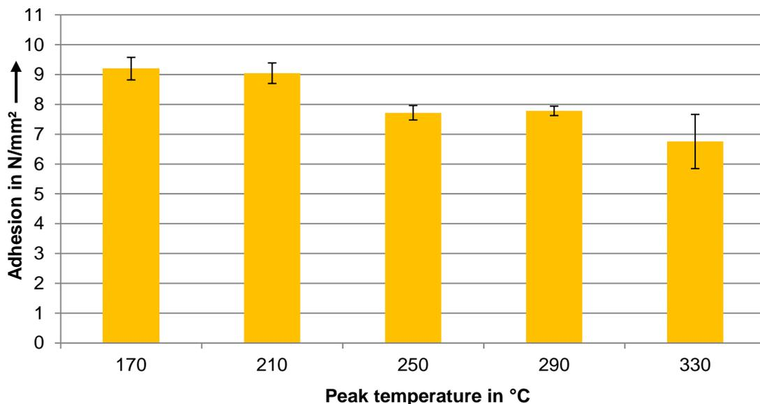
Fig 5: Evaluation of the hot pin pull test for temperature profiles with different peak temperatures
