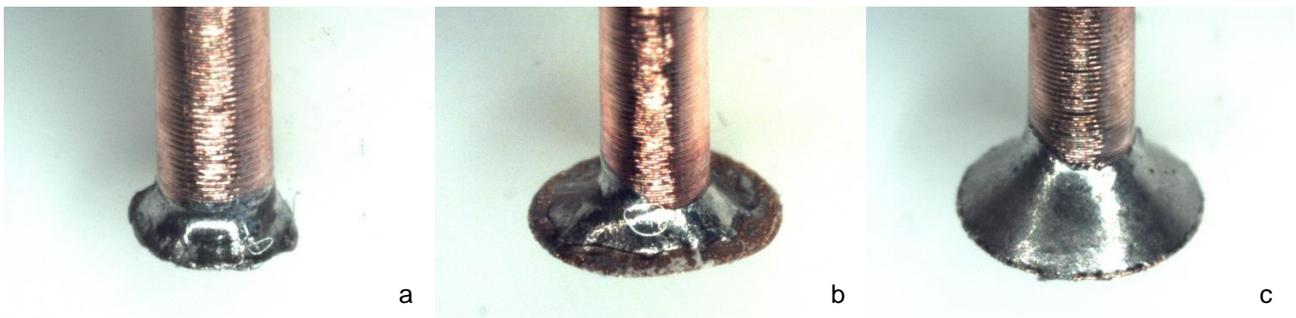
Fig. 6: Released test pads after the hot pin pull test with different solder wetting
