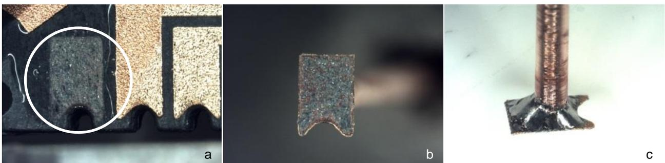
Fig. 7: Exemplarily illustration of pin and pad after the hot pin pull test
