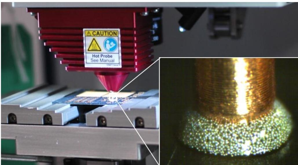
Fig. 2: Hot pin pull test with untinned pins
